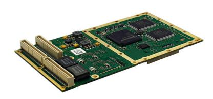
The P522 is a 32bit/33MHz PMC module with AFDX®/ARINC-664 functionality. AFDX® is a reliable, high-speed data bus commonly used in airborne applications for sending information between avionics subsystems. Its most important features are high data integrity, redundancy and deterministic behavior.
