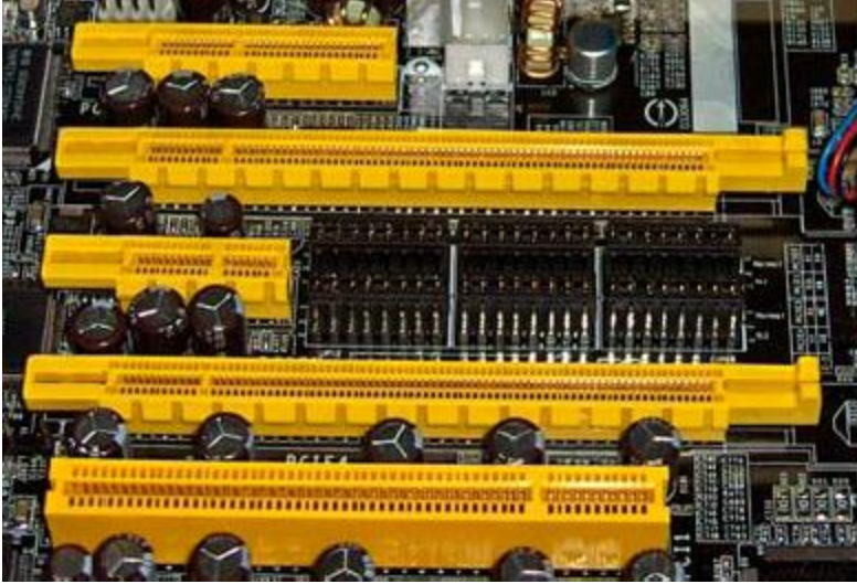
Figure 3: PCIe slots (from top to bottom: 4x, 16x, 1x and 16x), compared to a traditional 32-bit PCI slot (bottom)
