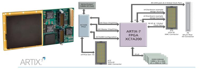
XMC module with PCIe interface ◆ Logic-optimized Artix-7 FPGA ◆ Write-protected flash
